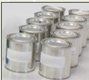
Figure 1. Unsaturated polyester paint blend samples
