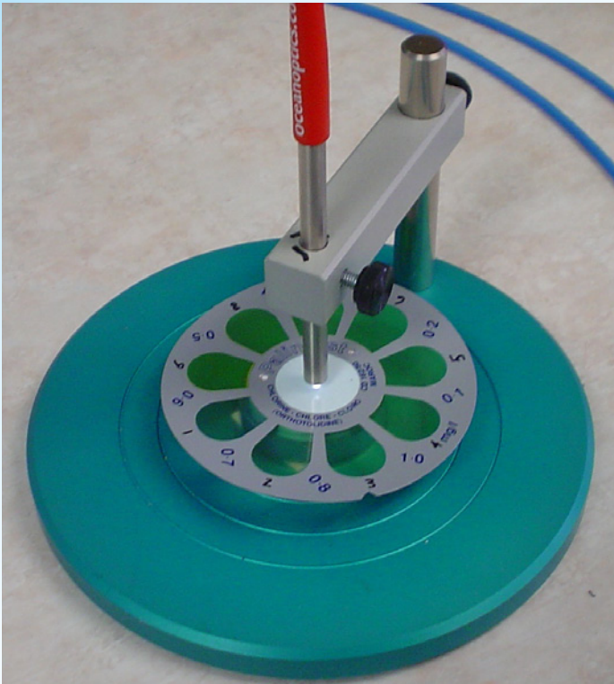
Figure 1: Spectroscopic measurements are useful for evaluating characteristics of a chlorine color wheel.
