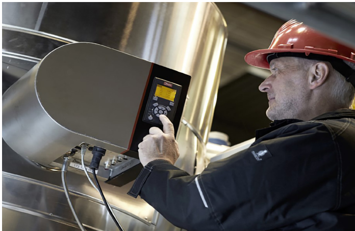
Figure 1. An Ocean Optics spectrometer assembly has been integrated into a maritime emissions sensor for use at sea.
