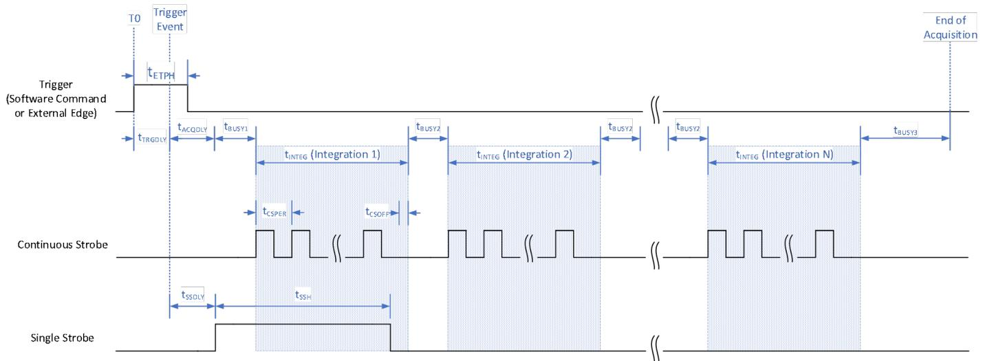
**Figure 3** – High Speed Averaging Mode Timing Diagram
